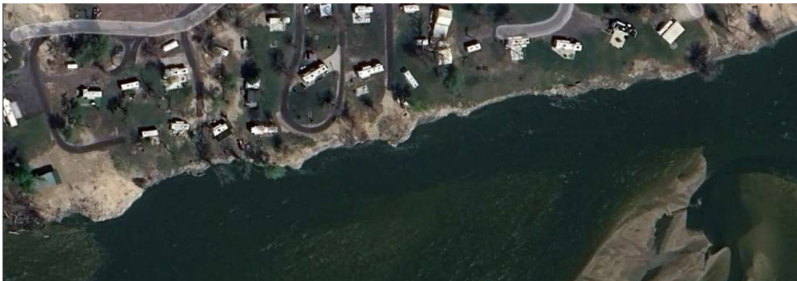
Figure 6: Example of Platte River Shoreline Armoring and Downstream Scour
